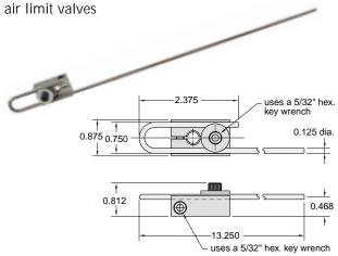
Arm: Steel 1/8" rod 13 inches long retained by screw clamp; the rod may be shortened and/or bent to desired shape
